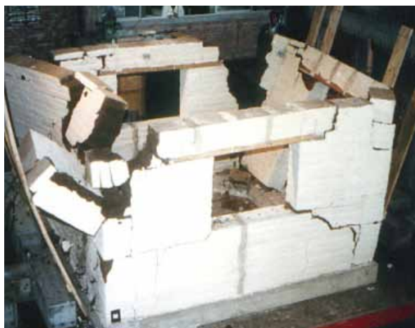
Figure 3: Testing adobe modules on a vibrating table. Top: module without reinforcement. Bottom: module with reinforcement
