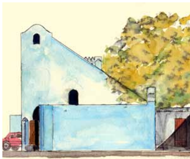
Figure 5: Eco-lodge prototype 'G' for Mr AbdAllah Schleifer, Tunness, Fayoum oasis. Egypt. 1992-93. The redundancy of the Eastern façade is because of the placement below to the left, of the access door to the septic tank concealed by the intentional end concavity of the wall screening the Japanese garden. Behind the same wall is a large opening for viewing the limited surface, and carefully designed walled Japanese garden. © Ahmad Hamid Architects
