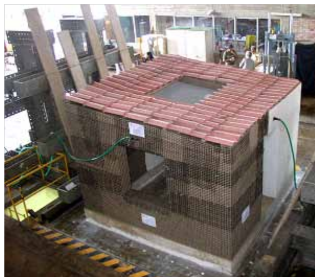
Figure 4: Module reinforced with a synthetic mesh or geogrid. Total area reinforcement, with half the module plastered. © J. Vargas-Neumann
