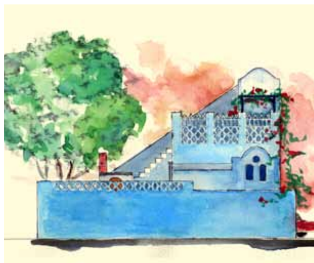
Figure 3: Eco-lodge prototype 'G' for Mr AbdAllah Schleifer, Tunness, Fayoum oasis. Egypt. 1992-93. Western façade rendering in watercolor (by Mr Seif El Rachidy) showing the multiple walled envelopes to the core space of the eco-lodge prototype. © Ahmad Hamid Architects
