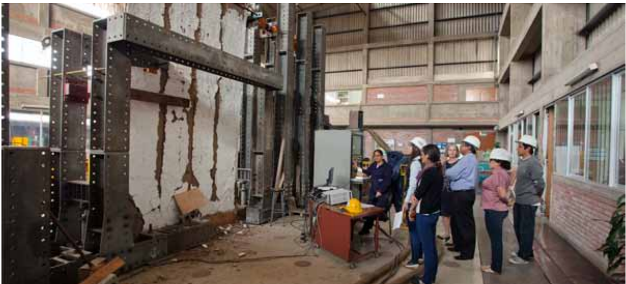
Figure 13: Wattle-and-daub ( quincha ) walls being tested to analyze their seismic behavior at PUCP. © Scott Warren, The J. Paul Getty Trust.
