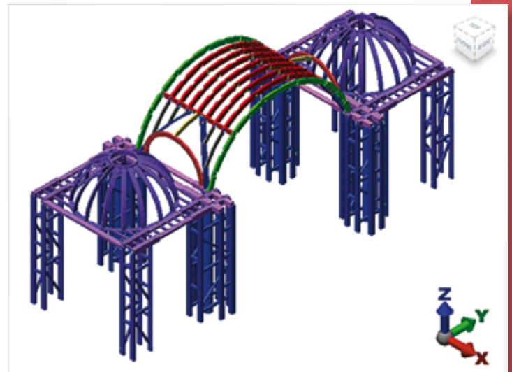
Figure 11: Partial numerical model of a representative bay of the nave and side aisles of Ica Cathedral, where the most important timber joints are simulated using realistic stiffness values obtained during the experimental campaign performed by PUCP. © Image and model: Carina Fonseca Ferreira, UCL, The J. Paul Getty Trust, 2013
